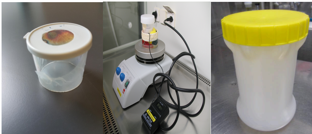
Figure 8: Enclosed feeding device system for Culicoides ; primary container “feeding chamber” (left panel) where live Culicoides will be kept during blood meal; secondary container, “infectious blood reservoir chamber” (middle panel) in a water bath and magnetic stirrer with temperature probe, and a transport box (right panel) for movement of the containers (feeding chamber and blood meal container) between rooms
