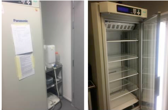
Figure 3: Example of an environmental/climatic chamber with humidity, temperature and light control. As depicted on the left panel, the chamber is connected to a water container for water supply and to a waste container to collect the waste water.
