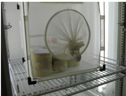
Figure 13: Containers with mosquitoes (sealed with mesh) in meshed cage inside environmental chamber.
