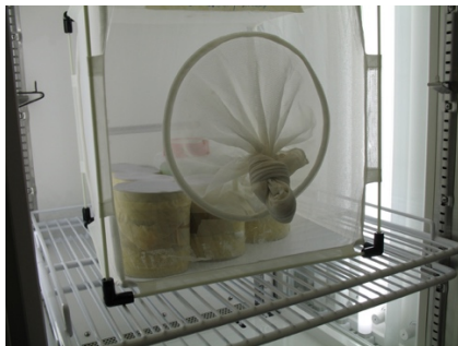
Figure 13: Containers with mosquitoes (sealed with mesh) in meshed cage inside environmental chamber.
